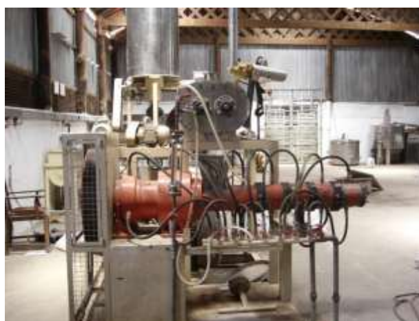
Figure 4 An Extruder: Sigma Feeds Nairobi Kenya, producing floating feeds for the Kenyan aquaculture industry now opening up opportunities for commercial cage culture across the country
